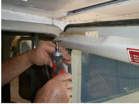
Figure 2. Slotting Plastic with Dremel
