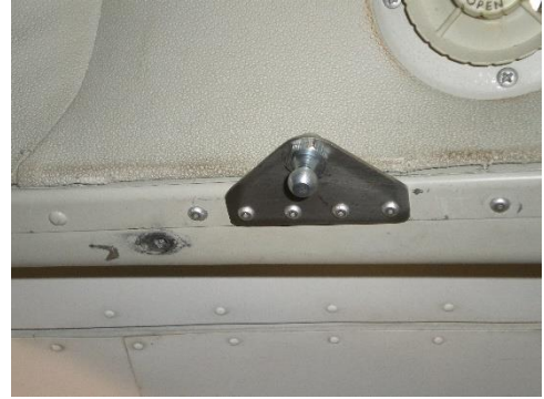
Figure 7. Airframe bracket installed
