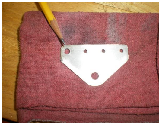
Figure 1. Hole enlarged in one of the brackets.
