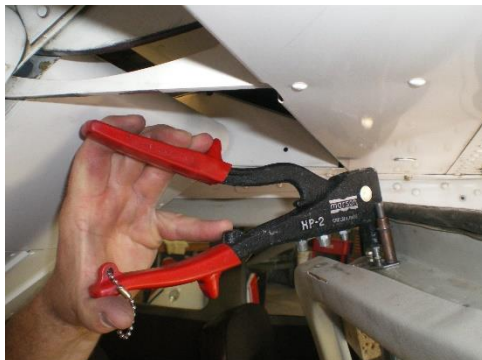
Figure 4. Riveting bracket in place
