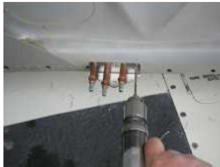
Picture 5. Drilling Door Bracket
