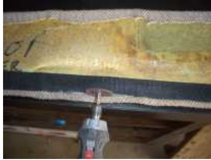
Picture 7, Slotting Interior panel on Baron.
