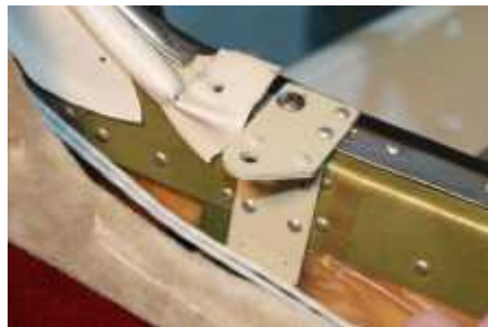
6. Airframe bracket attached (Note: bottom 2 pilot holes not used)
