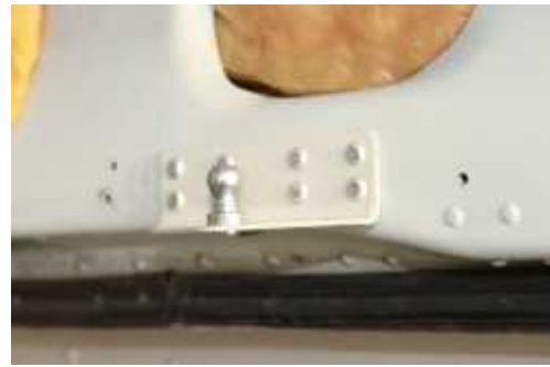
9. Door Bracket installed
