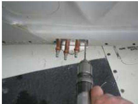
Picture 5. Drilling Door Bracket
