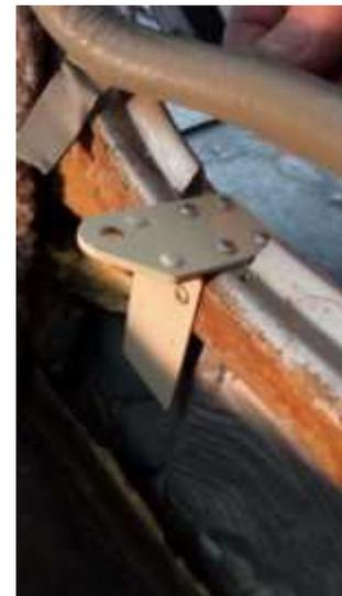
8. Install the door bracket, P/N 201C103-2 inverted on the door in a position that will be not less than the 10" dimension as depicted in the picture with the door closed and approximately 1" above the bottom of the door. Angle the bracket slightly to align with the airframe bracket.
