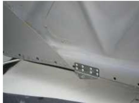
Picture 6. Door Bracket Installed
