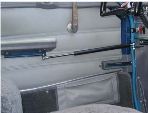
Picture 4. Installation Complete Door Closed
