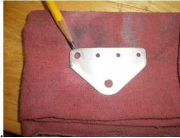
Picture 1. Hole enlarged in one of the brackets
