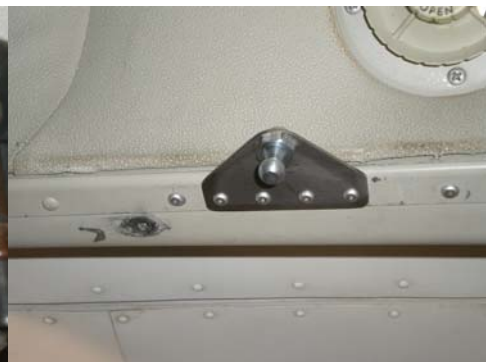
Picture 6. Distance from slide attach hole Picture 7. Airframe bracket installed
