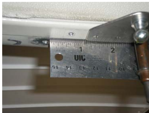
Picture 6. Distance from slide attach hole Picture 7. Airframe bracket installed
