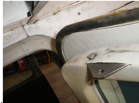
Picture 4. Riveting Bracket in Place. Picture 5. Complete Door Bracket
