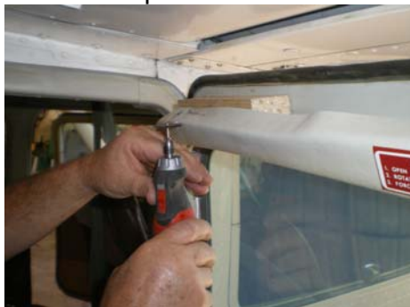
Picture 2. Slotting Plastic with Dremel Picture 3. Drilling #30 holes.
